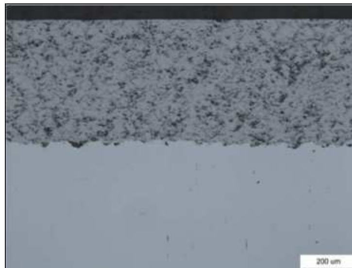
FIGURE 29 - OVERVIEW OF SUPPLIER "E" COATING
