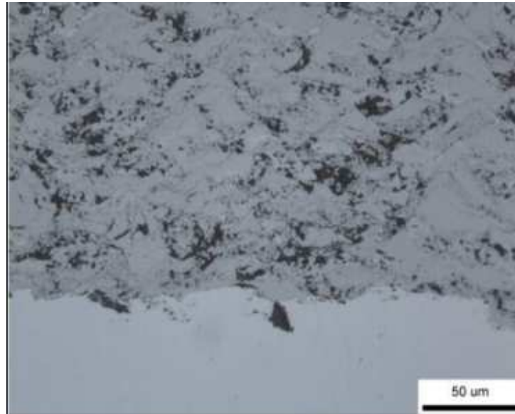
FIGURE 30 - DETAIL OF SUPPLIER "E" COATING
