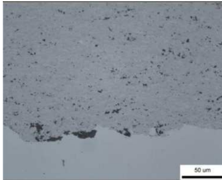
FIGURE 18 - DETAIL OF KERMETICO COATING
